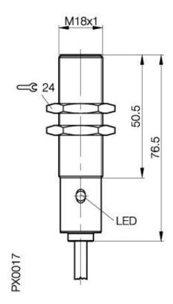
**Inductive Sensors** BES 516-111-BO-C-PU-05 M18x1 x 76.5 Complementary Sn=5mm shielded
